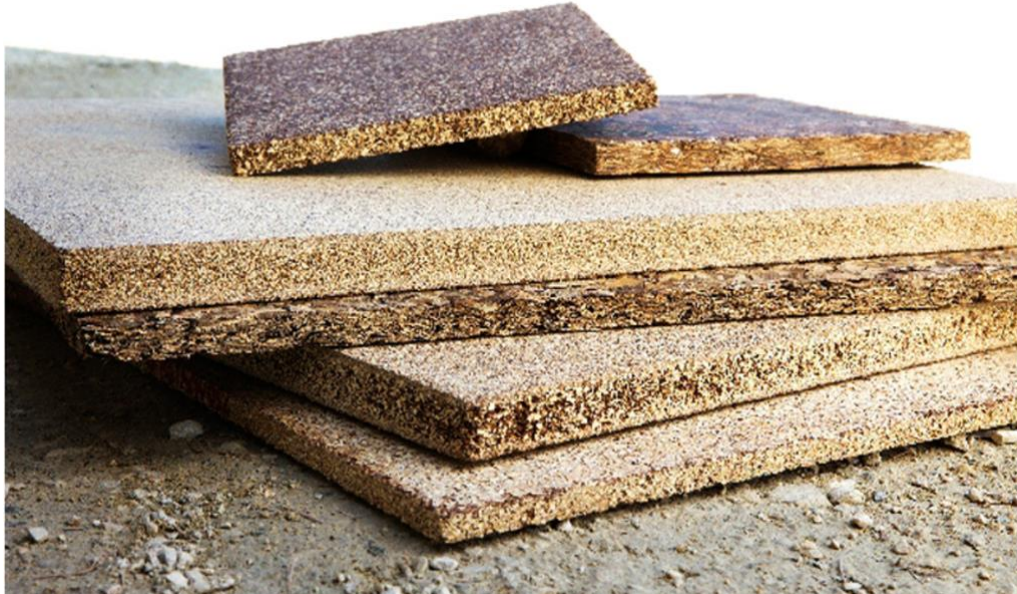
Figure3-17: Composite panel produced with organic waste [47]
